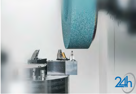
Automatic mill dressing with dimensional tool compensation.
